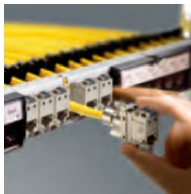
Simple unclipping of LCS 2 connectors
