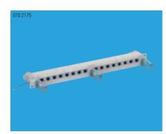
For smaller distributors, the use of 19" 1U patch panels is recommended. Up to 16 shielded or unshielded single RJ45 connection modules can be installed in the 19" 1U rack, which corresponds to a maximum connection density of 16 RJ45 ports. Thanks to jumpering brackets the line and patch cords can be neatly arranged at the side of the rack.
